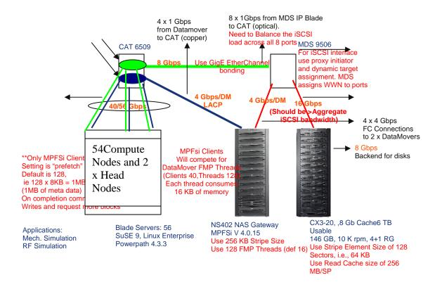
**Fig 2: Production Setup**
