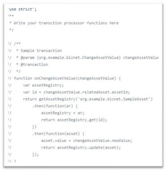
The following code snippet is an example of a very basic logic.js file adapted from a file storage GitHub repo on the topic of blockchain and file storage<sup>(19)</sup>.
