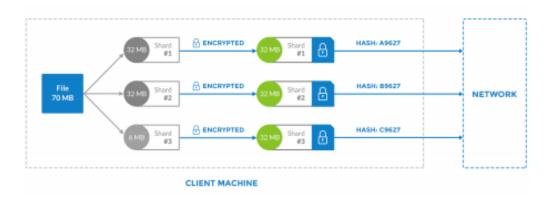
The diagram above illustrates the sharding process on each client adapted from the *Storj - A Peer-to-Peer Cloud Storage Network Whitepaper.* Each client is holding secured information which is auditable across the network through smart contracts. This is able to be achieved through two proprietary protocols: Proof-of-Storage and Proof-of-Redundancy<sup>(8)</sup>.
